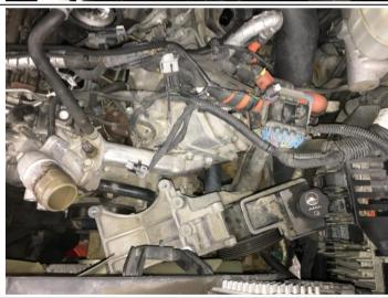
Remove oil fill tube, then thermostat housing with crossover and bypass pipe.
