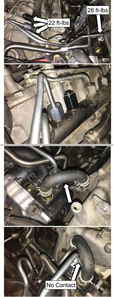
Remove indicated high-pressure line mount and clamp from original lines.
