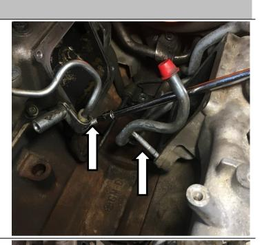
If necessary, adjust crossover and return lines to not contact CP3.
