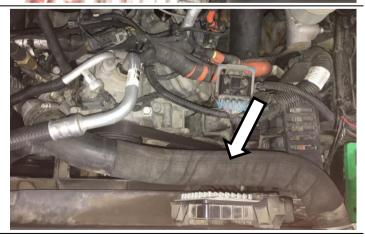
Reinstall two intake manifold studs removed earlier.
